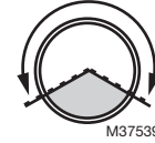
Fig. 2. Meter installation range for horizontal pipe.
